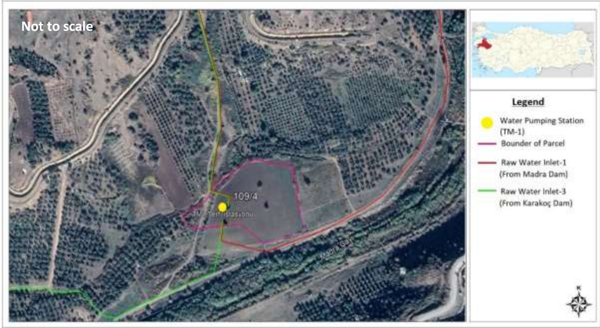
Figure 4.2 Land to be acquired for the Raw Water Pumping Station (TM-1) 3
